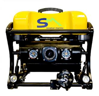
The **CHINOOK** is an industrial grade inspection ROV with a wide range of capabilities. Explore depths of 300 m (1,000 ft) with the standard vehicle or 600 m (2,000 ft) with the deep water version.
